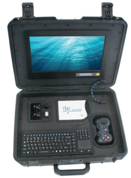
Surface Control Unit
